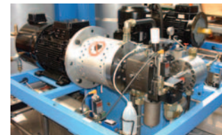
Maintenance-free sealing of dosing pump for polyde and isocyanate in high-pressure reaction casting machines
